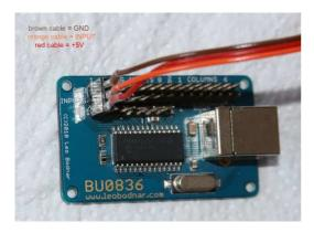
So, if all sensors are connected, all red wires must be are on the same side corresponding with the [+5V] label.
